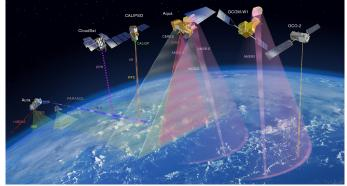
★ Aura MLS has radiometers in 5 broad spectral bands centered near 118, 190, 240, 640, and 2500 GHz (wavelengths from 2.5 to 0.1 mm)
